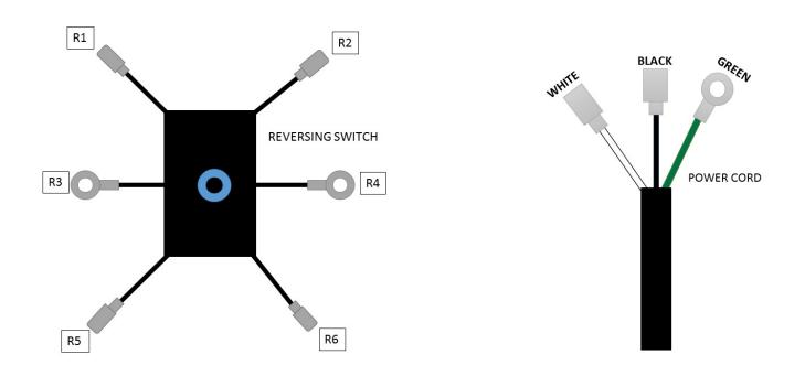
REVERSING SWITCH TO MOTOR: R2 to Red (Tape)
