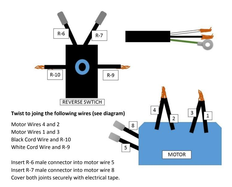
Using wire nuts, join the following: Motor Wires 4 and 2 with white cord wire and R-10 Motor Wires 5 and 8 with black cord wire and R-9
